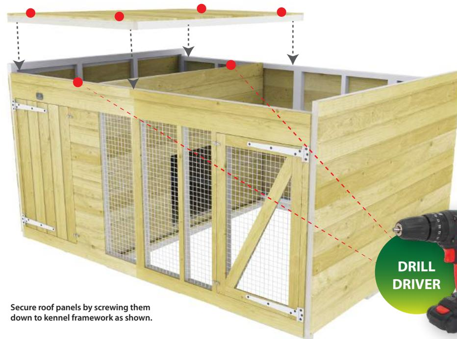
Secure roof panels by screwing them down to kennel framework as shown.
