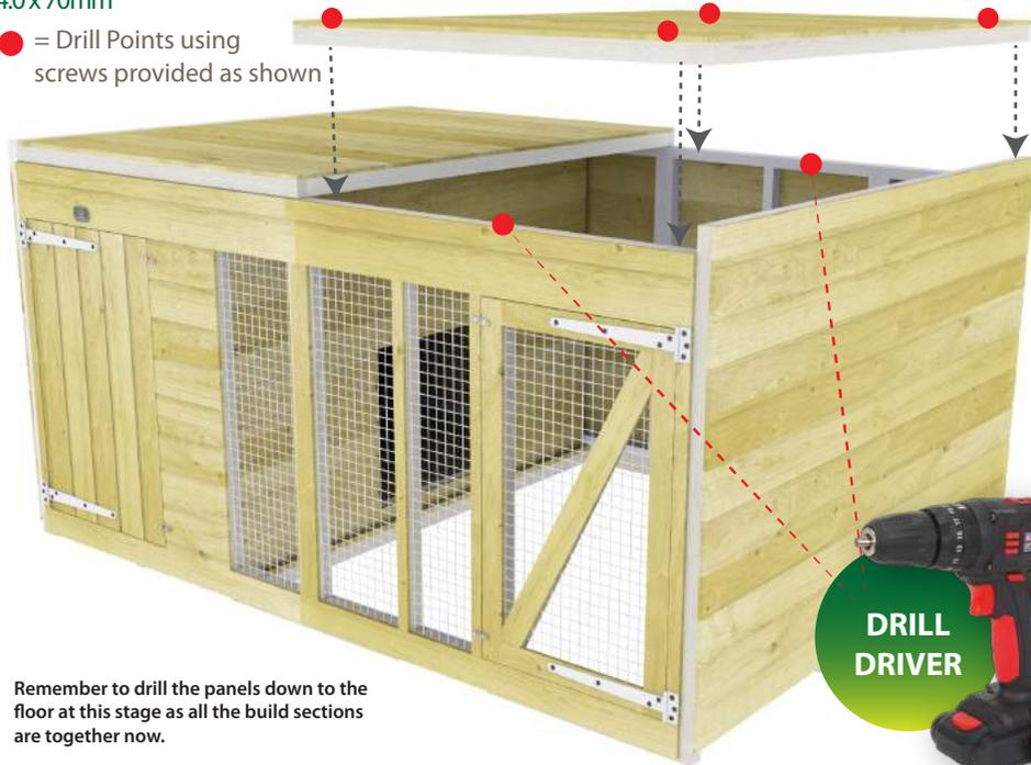
Remember to drill the panels down to the floor at this stage as all the build sections are together now.
