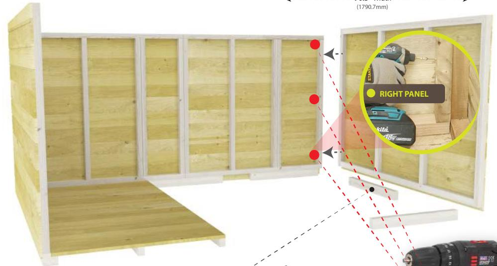
Use 12" Floor Block Posts elevate the right side panel and screw in sides to secure against the 2nd back panel side post as shown.
