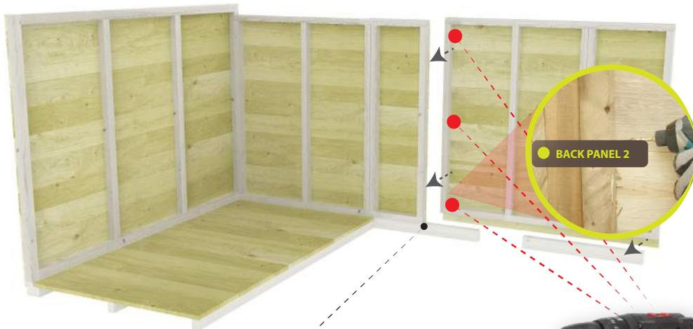
Using the Floor Block Post to elevate the 2nd back panel and screw in sides to secure against the 1st back panel side post as shown here.
