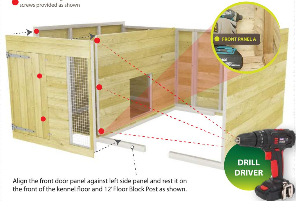
Align the front door panel against left side panel and rest it on the front of the kennel floor and 12' Floor Block Post as shown.
