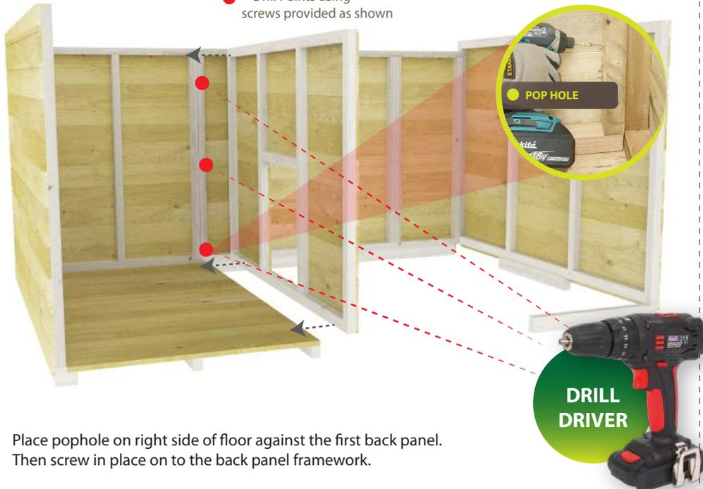
Place pophole on right side of floor against the first back panel. Then screw in place on to the back panel framework.
